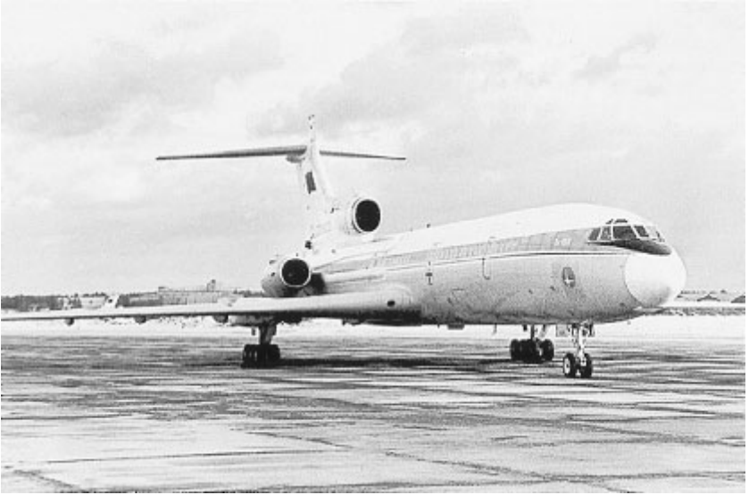
The Tupolev 154 passenger jet, with one engine converted to run on hydrogen. (courtesy of DaimlerChrysler Aerospace Airbus)
