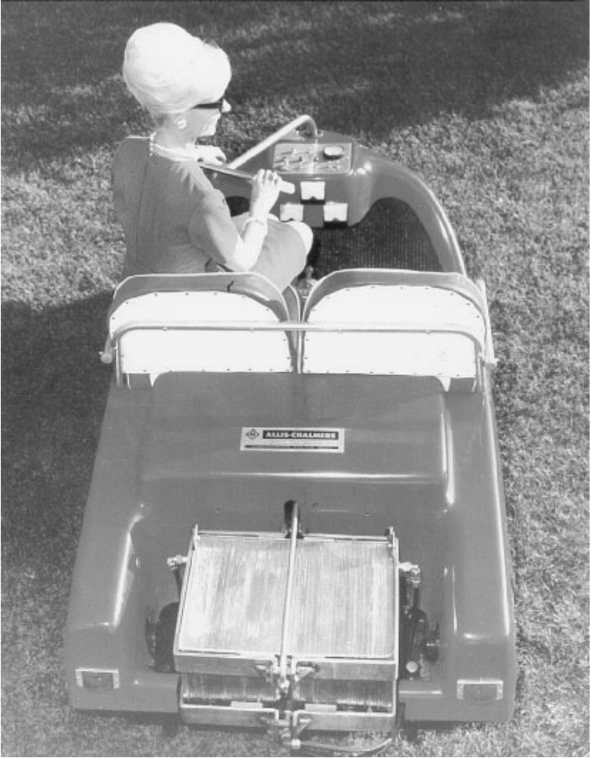
The experimental Allis-Chalmers fuel cell golf cart of the early 1960s. (courtesy of Jay Laskin)
