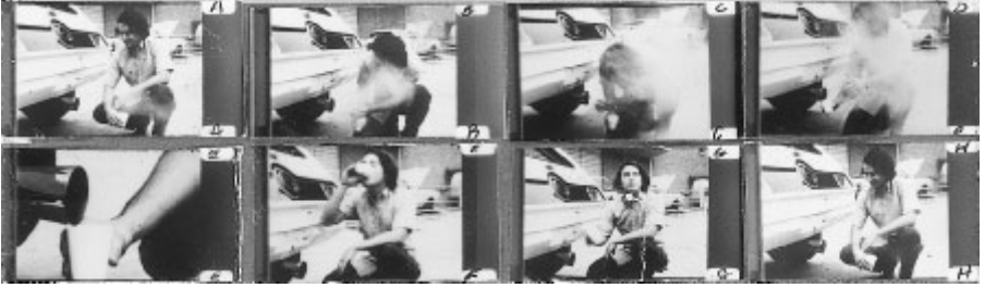
Ned Baker, a member of the 1972 UCLA Urban Design Vehicle Competition team, graphically demonstrates the cleanliness of an engine fueled by hydrogen. The almost pure water he is drinking condensed out from the steam coming out of the tail pipe. ( prints from 16-mm film clip produced by UCLA )
